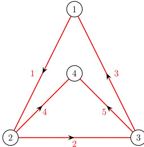
A circuit is represented above by a directed graph with four nodes in black and five edges in red. Electrons flow from one node to the other if the voltages (or electric potentials) are different. The unknowns are:
